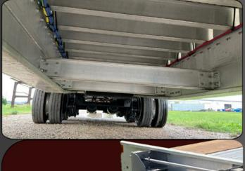
The Chaparral II Tag trailer series uses the same aluminum main beam, crossmember, and side rail extrusions that have been used in the Chaparral II Class 8 drop deck trailers since 2013.
