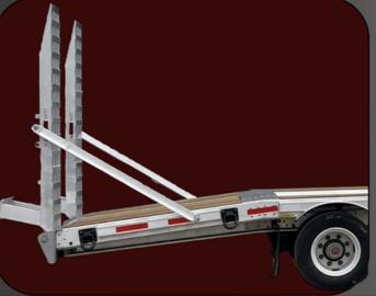
Doonan utilizes custom aluminum ramps to achieve an 8-degree angle providing for easy equipment loading and unloading. The spring assisted light weight ramp is extremely easy to Lift, Lower and Slide side to side minimizing any potential injury to operator.
