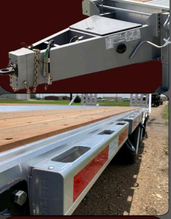
Doonan replaced the steel gooseneck used on its Chaparral II drop deck trailers with a galvanized steel A-frame pintle hitch (tongue /drawbar) to providing unmatched corrosion protection.
